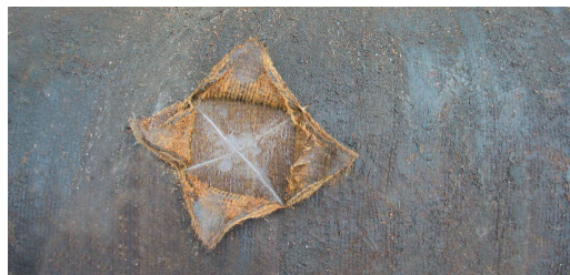
An inspection of the pipe revealed the surface underneath the tape to be in excellent condition with no corrosion.
