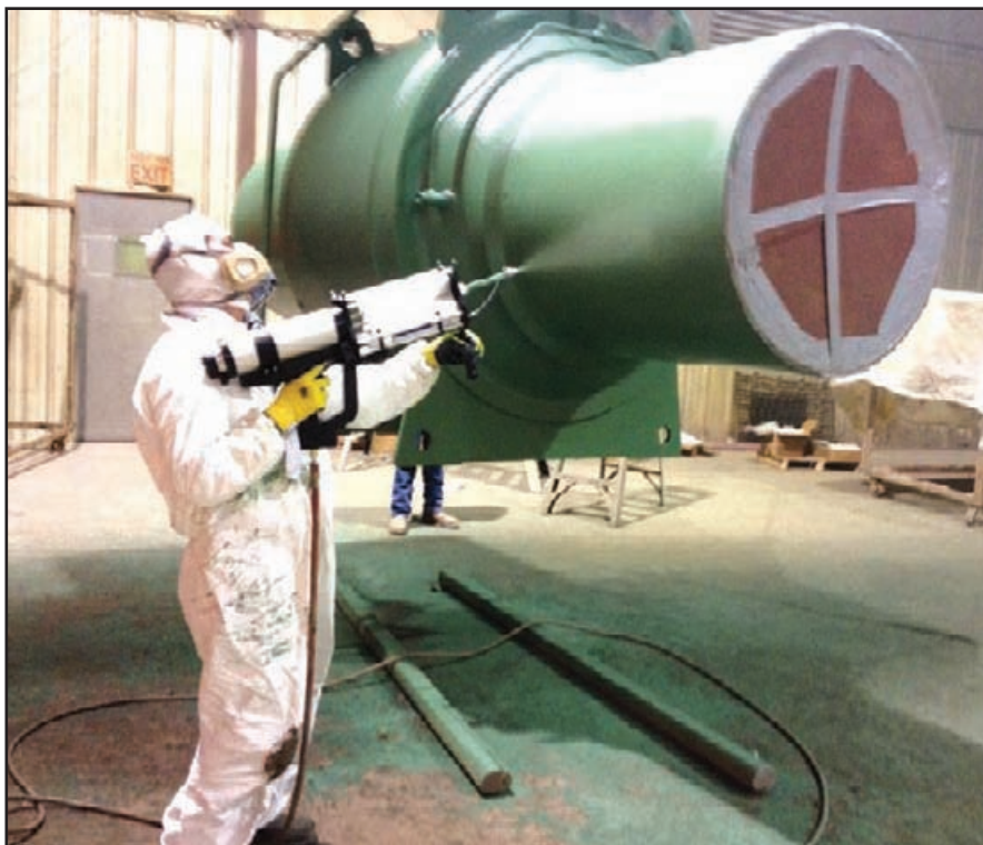
Above: The Protal 7200 Air Cartridge Gun.
