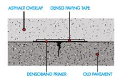
A cold applied, fabric re-inforced, polymer modified bitumen membrane for sealing up to 5mm wide in asphalt and concrete road pavements prior to overlaying with asphalt.
