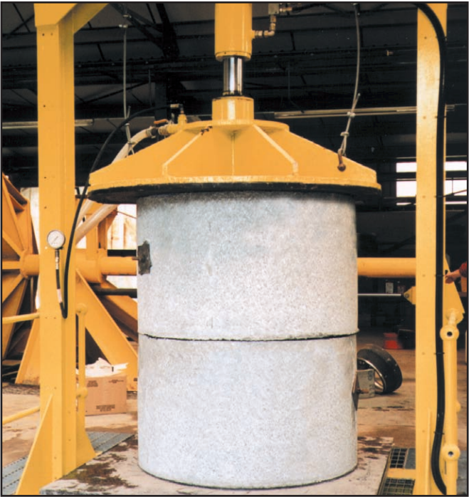
Independent water pressure testing of manhole units joined with Densostrip to determine seal strength.
