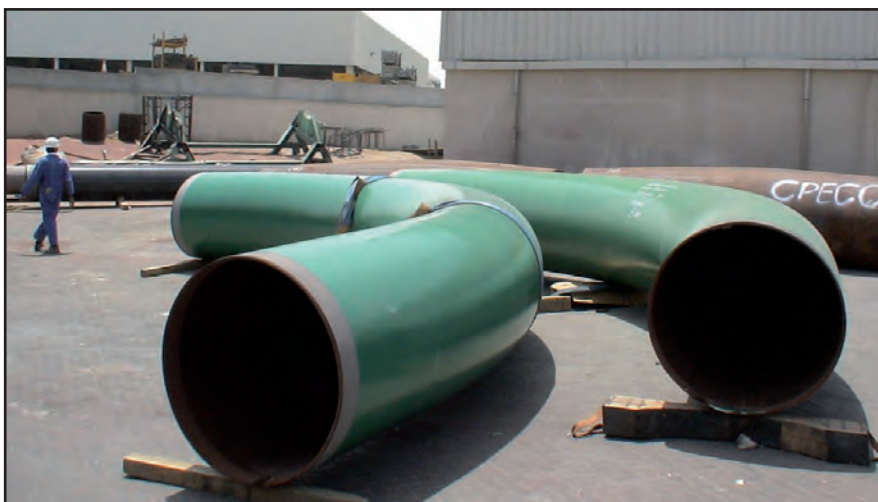
Above and Below: Pipe lengths coated with Denso Protal 7200 prior to installation on site.
