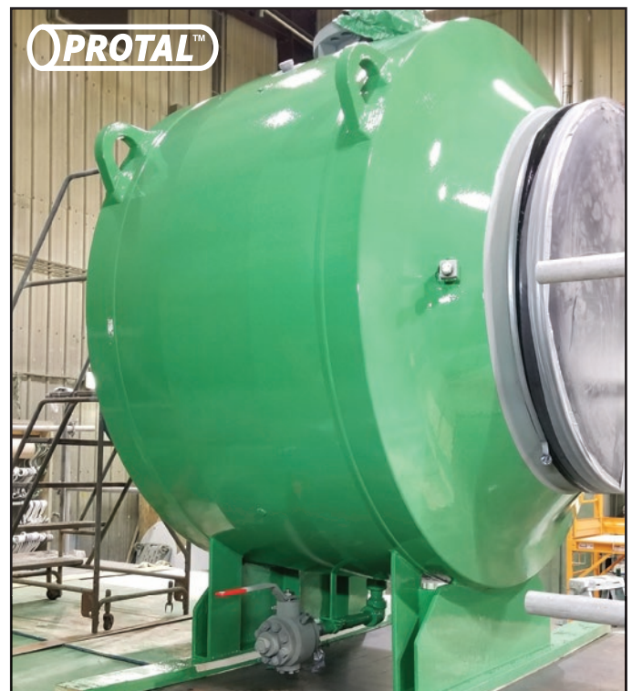
The valve is finally coated with Denso Protal 7200™.
