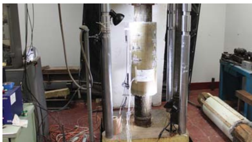
Compression testing of timber piles.
