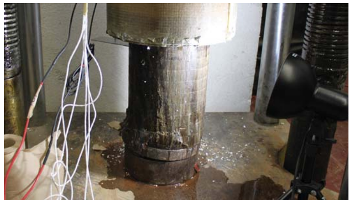
SeaShield Series 400 System repair not only restores the original axial capacity of the pile but also enhances it by 3% to 22%.
