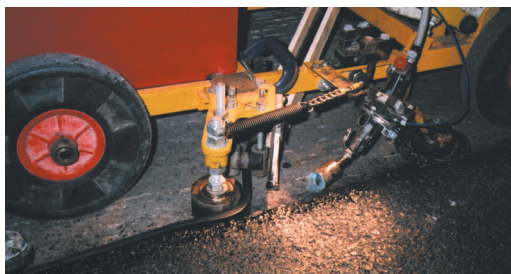
Close up of the Densoband™ applicator machine.
