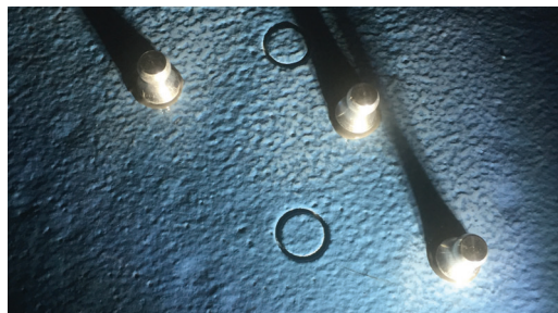
Adhesion test, 2500 psi to 2800 psi
