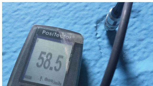
System 400 primer @ 4 to 5 mils dft, 30 to 35 mils dft of 476F single leg.
