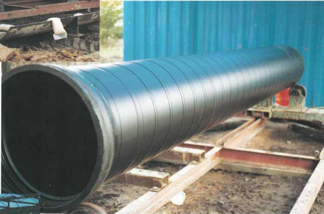
The end product - a tight, tough, uniform tape coating.
