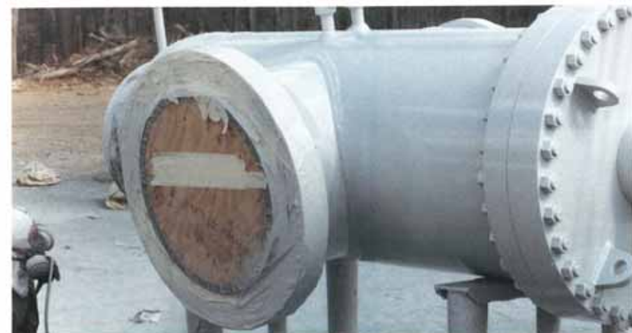
Large valve being spray protected with Protal 5900 prior to shipment to field.
