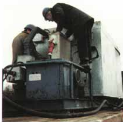
The special Denso Void Filler pumping system.
