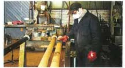
Surface of tie-bar is first cleaned.
