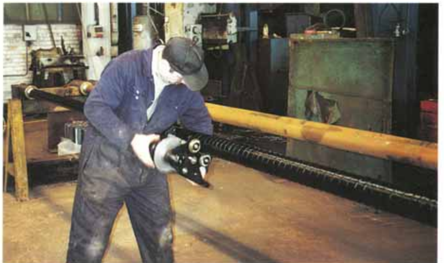
Densopol Tape is applied by hand operated Densoman machine achieving fast uniform wrapping.
