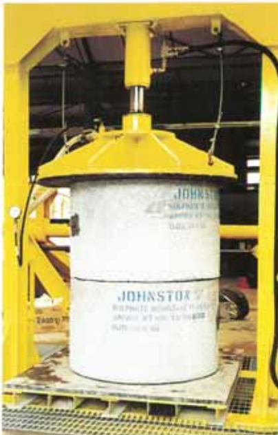
Above: Independent water pressure testing of manhole units jointed with Tokstrip to determine seal strength.
