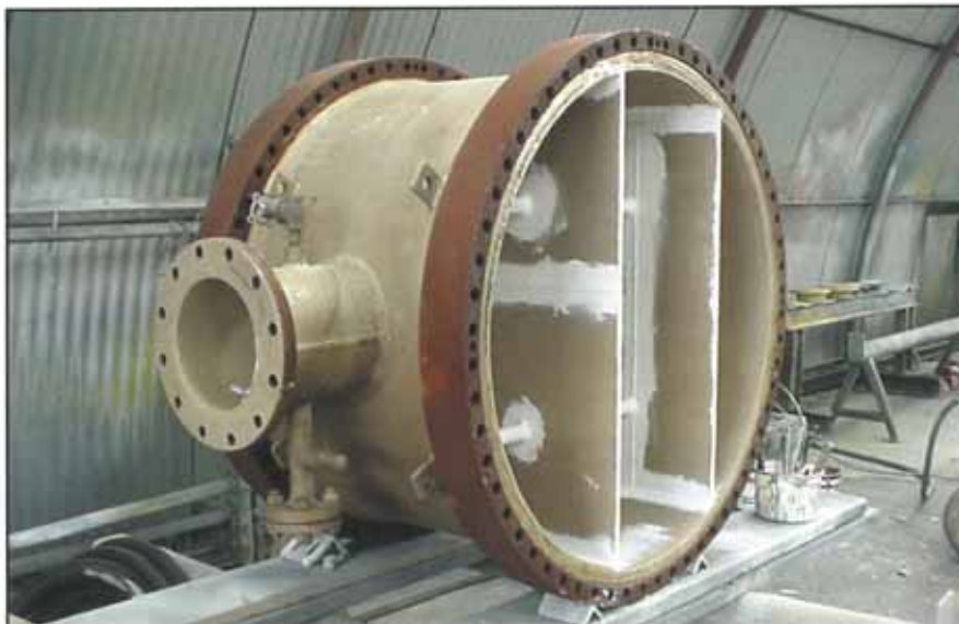
Above: Stripe coating of flange underway. Below: Completed Archco-Rigidon coating protection.
