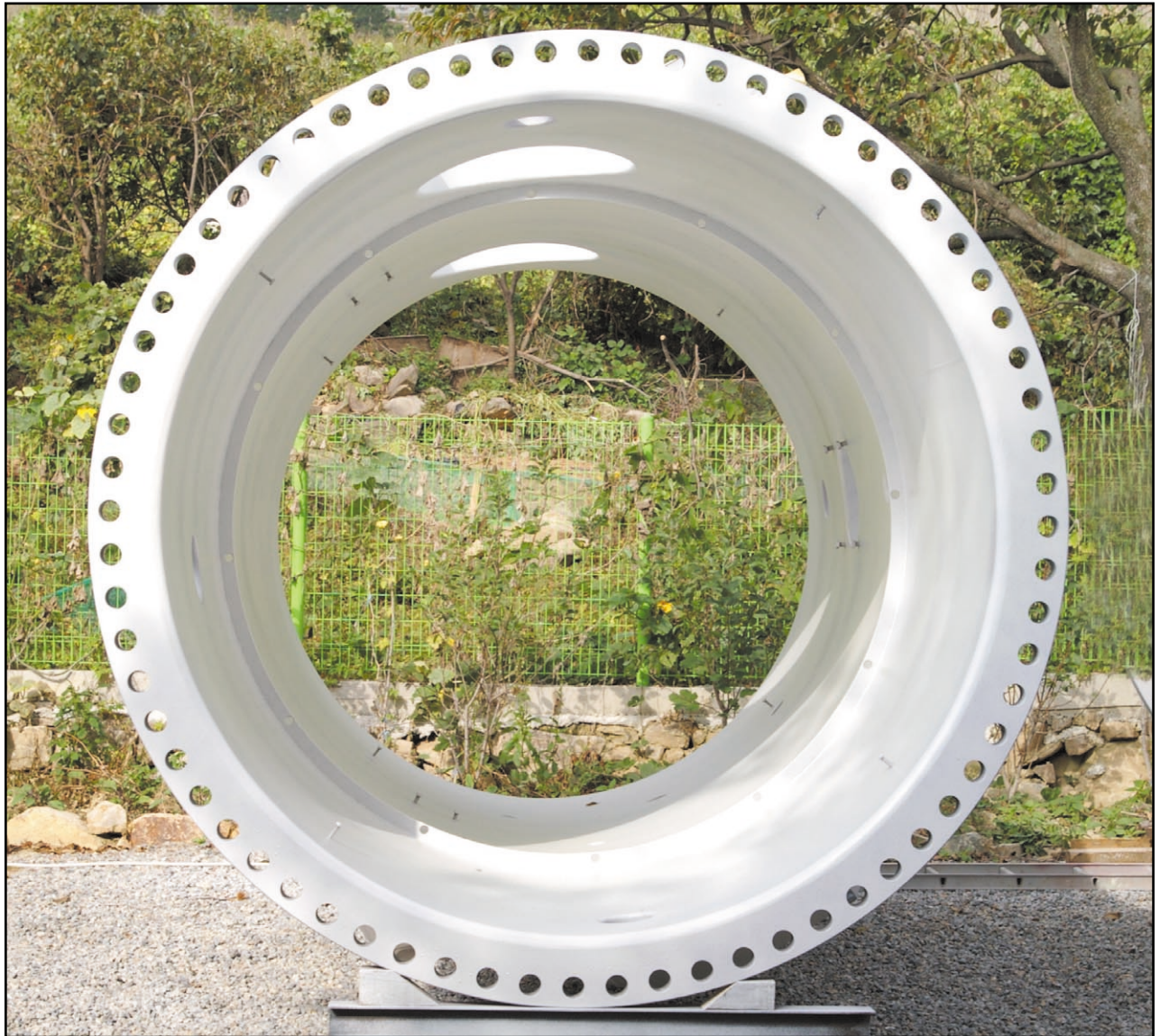
Archco-Rigidon Rigspray lining protects Korean nuclear plant debris filter - see story page 8.
