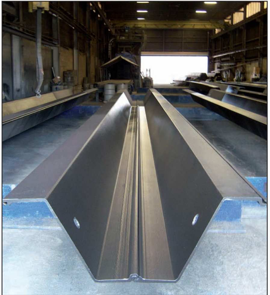
Above: New sheet pile just after Rigspray was applied (55" wide x 45' long weighing over 6,000 lbs.)
