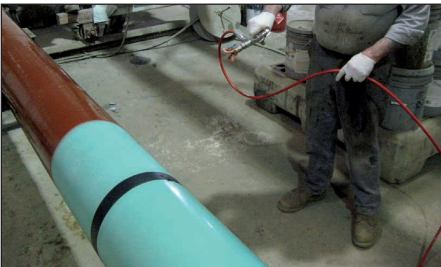
Photos: Above: Directional drill application with Protal ARO coated pipe. Below: Protal ARO being spray applied in the shop
