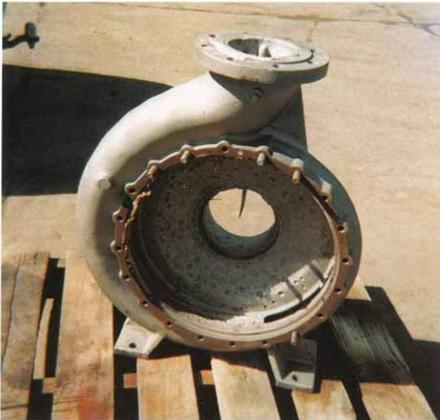
A grit blasted pump coated with PD-2 Primer.
