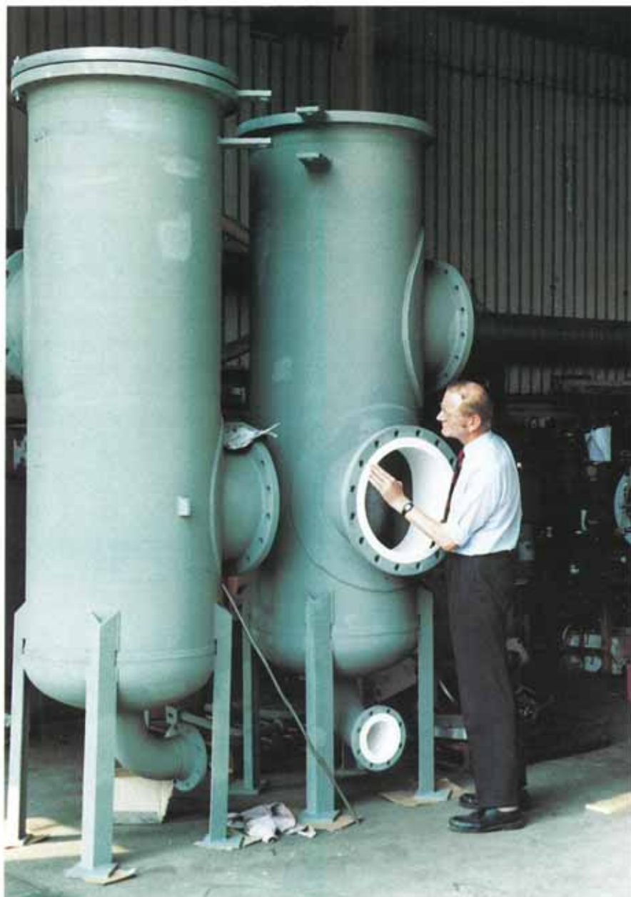
A pair of sea water filter vessels built by Plenty Ltd and protected with Archco-Rigidon 423D.
