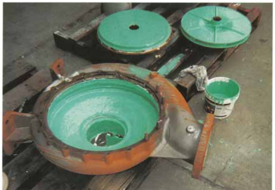
Pump components coated with the final coat of Archco-Rigidon 423D which is in a contrasting colour.
