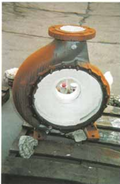
The white base filler coat of Archco-Rigidon 423D.
