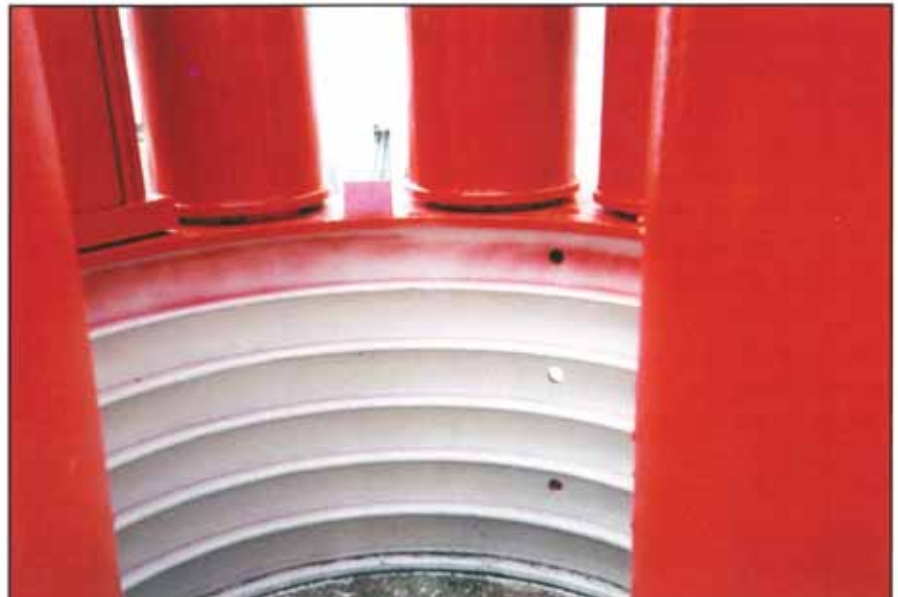
Above and below: Denso S.T. Epoxy coating used on the 'Katja' jack up barge.
