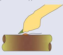
2. Clean the area to be coated with cleaning wipe. Remove any loose particles, grease, debris or moisture. The area should be clean and dry. Please refer to the Viscotaq Technical Manual for full surface preparation requirements.
