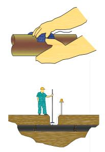
6. Viscotaq Coating Patch comes with Velcro dot for use at keyhole applications.
