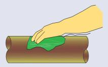
3. Remove Viscotaq Coating Patch from packaging and peel off release liner.
