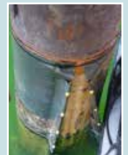
The weight loss coupons at the two control pile locations were fitted outside of the installed pile wrapping and sleeving system to enable "real time" corrosion rates to be calculated to compare against those corrosion rates experienced below the tape and sleeve systems.
