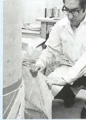
High bond is apparent as many fibers remain embedded in FX-70-6 Hydro-Ester mortar.
