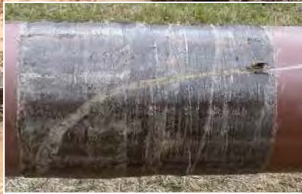
Above: Denso Bore-Wrap® shown to have protected the underlying coating after bearing failure.
