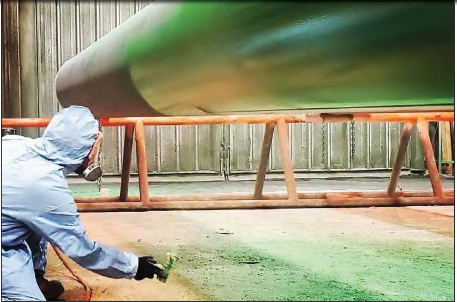
Above: Plural Spray Application of Protal 7200.
