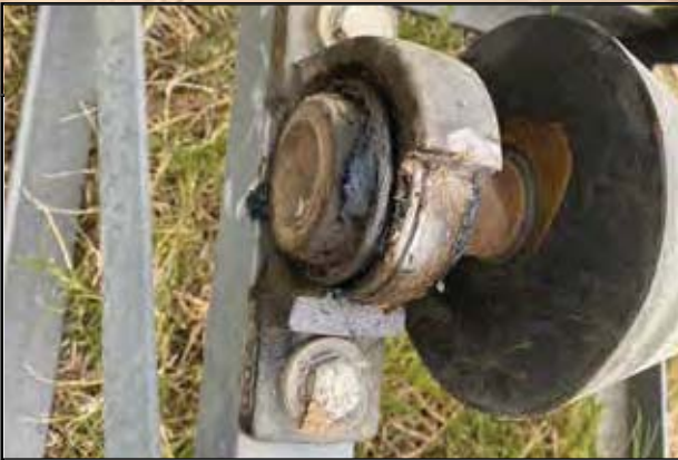
Failed pipe roller bearing.
