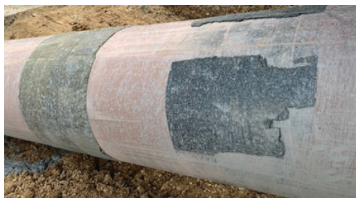
The Denso Bore-Wrap is fully intact on the left after the pull.
