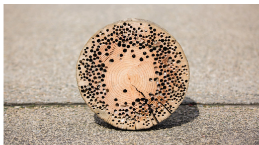
Marine borer damage to timber piles.
