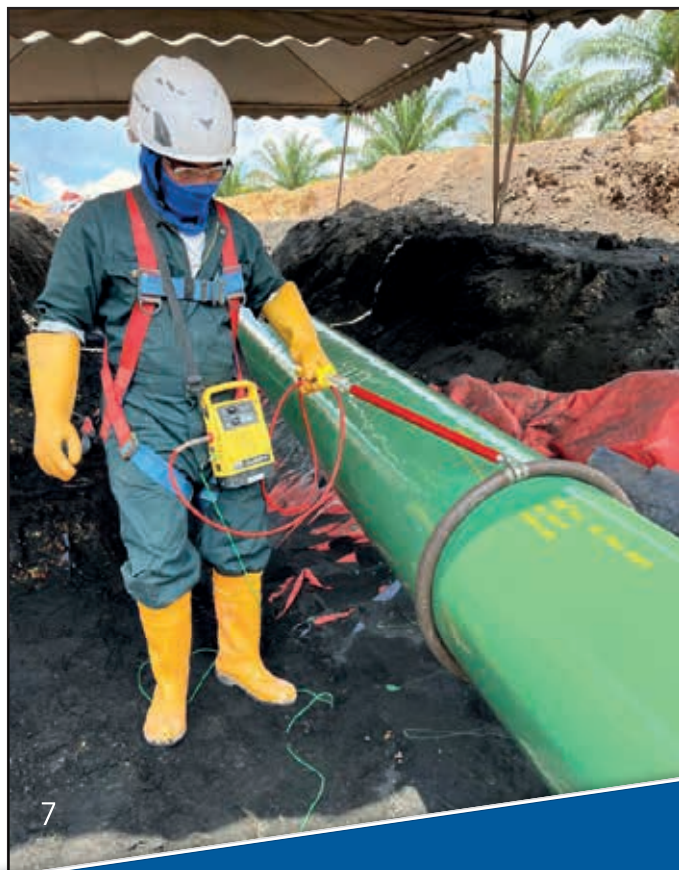
Below & right: Holiday testing of the cured Protal 7200.
