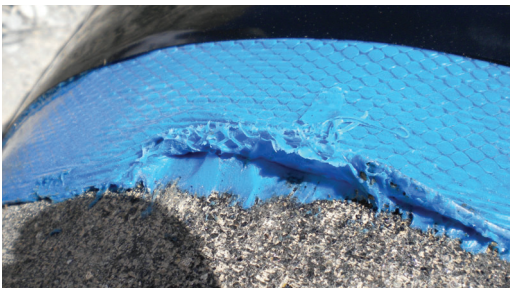
The ViscoWrap HT shows strong adhesion to any of existing pipeline coatings.
